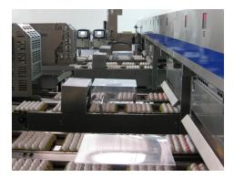
CIJ printers installed on grader
