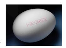
The vast majority of eggs being coded today are coded with red, ink-based systems, because inks do not alter the integrity of the egg. The food safe inks are formulated to adhere to the shell. The inks typically dry in a couple of seconds, and once dry, are resistant to water.
